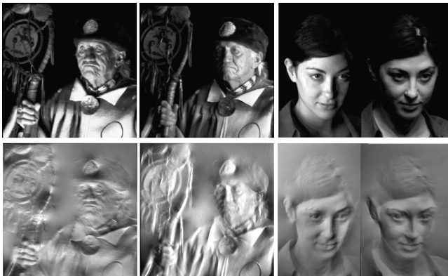
Figure 7: Pairs of images taken under different illumination conditions, resulting optimized simulated pair and photographs of the machined surface for roughly equivalent light directions.
